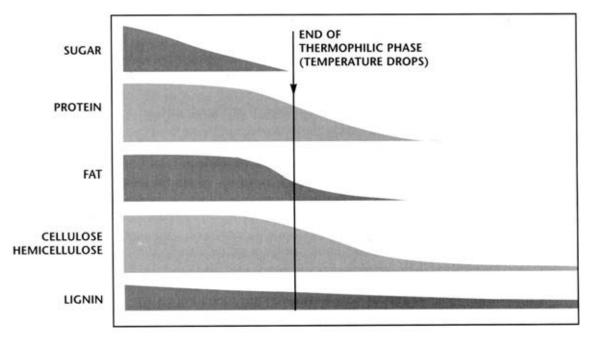
figure 2.7: chemical decomposition during thermophilic composting
