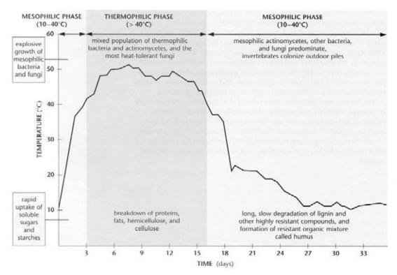
figure 2.6: the three phases of thermophilic composting
