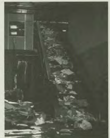
Paper conveyor at Somerset County MRF. Worker to left of conveyor is responsible for pulling any bags of textiles off of conveyor.
